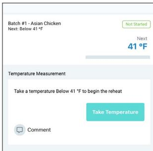
If you are taking a temperature with the SmartSense Probe, you will need to turn on the probe then tap **TAKE TEMPERATURE** on the mobile app screen. The probe will display the reported temperature on the mobile app screen, and once the probe has stabilized, select **SAVE**. If you are manually taking a temperature, tap the temperature box, enter the temperature using your keyboard, and select **DONE**. Tap **SAVE** to continue.
