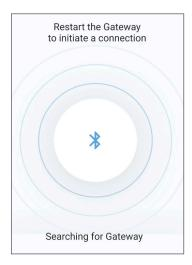
If you are unable to connect the gateway, make sure you have entered the correct ID then select the **RETRY** button. Restart the gateway using the steps above. When the gateway successfully pairs, you will automatically be redirected to the **GATEWAY CONFIGURATION** screen and see a blue banner showing that you have network connection.
