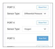
To the right of each port is a blue **SCAN PORT** button. When you click this button, the port will start scanning for a connected sensor. If the sensor is properly connected, select the appropriate **SENSOR TYPE** from the dropdown to assign it.
